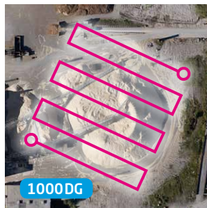
On the right, less flying is necessary with the Direct Georeferencing (DG) solution, which means less flight time, as well as fewer photos to process later.
