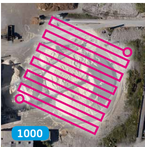
On the right, less flying is necessary with the Direct Georeferencing (DG) solution, which means less flight time, as well as fewer photos to process later.
